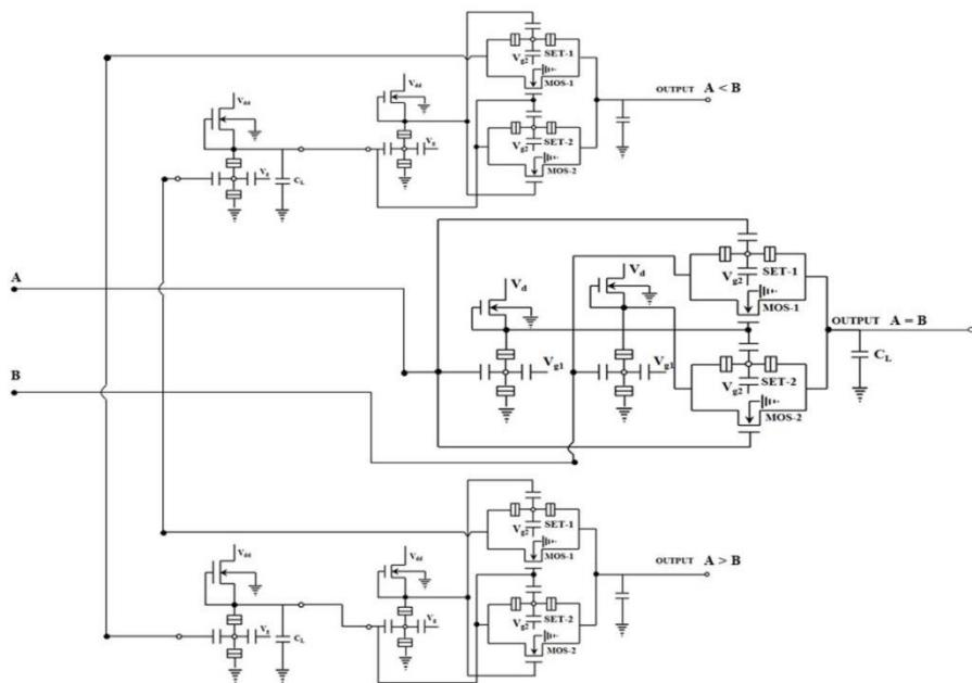
**Fig1:**Hybrid CMOS SET based Comparator
